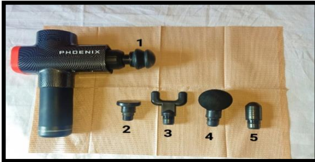
Figure 5 The handheld vibration gun device, with interchangeable attachment heads. The soft attachment head will be utilized in this study (1), Hard plain. (2), spinal (3), hard ball (4), and trigger point head (5).
